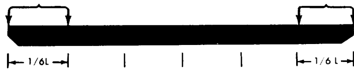
LOAD CONDITION A LOAD BEARING POINTS ON OUTER ONE-SIXTHS OF SKID LENGTH
